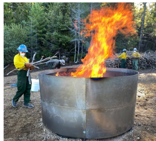
FIGURE 4: THE RING OF FIRE BIOCHAR KILN DESIGNED BY WILSON BIOCHAR ASSOCIATES. THE TOP LIT FIRE, LIMITS OXYGEN IN THE LOWER PORTION OF THE BURN, CREATING PYROLYSIS CONDITIONS. (LEFT: WILSON BIOCHAR ASSOCIATES) (RIGHT: DAVID MORRELL)
