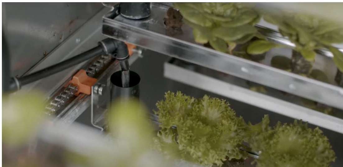
Figure 5. Irrigation system inside the machine for harvesting lettuce in “Cubicfarms” (Adapted from “Cubicfarms”. 2020)
