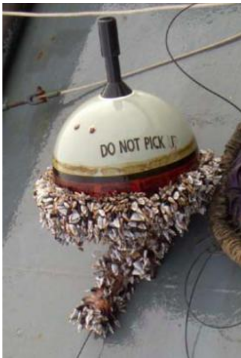
Appendix D-1 The situation of microorganism colonization of a 521 days floating spherical buoy (NOAA, n.d.).
