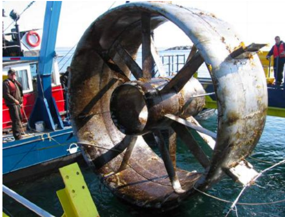
Appendix D-2 Six-month recording of fouling organisms on tidal turbines (Fletcher, 2007).
