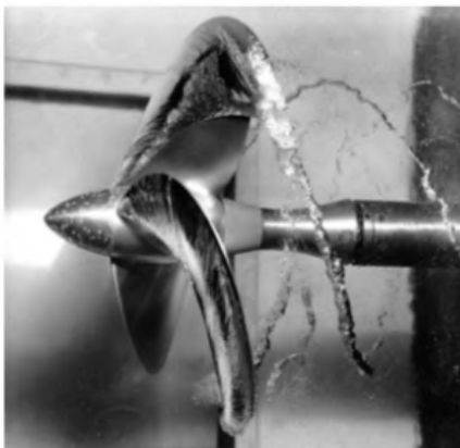
(c) Partial sheet cavity
